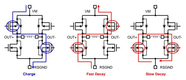
\* The TB67H420FTG has a 400ns (design value) dead time to avoid any flow-through current during switching.
