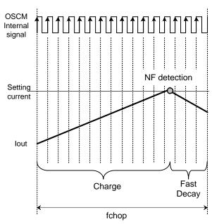
If NF detection is overdue, Decay sequence will only be Fast Decay.(Slow Decay does not appear.)
