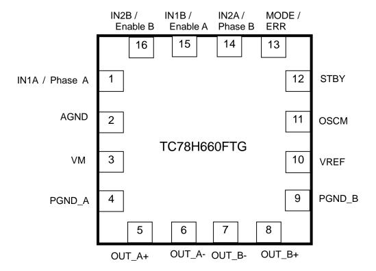
Note: Please solder the corner pads and the rear thermal pad of the QFN package, to the GND pattern of the PCB.
