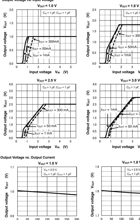
**Output Voltage vs. Input Voltage**
