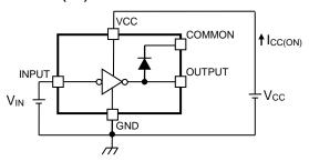
Test circuit and timing chart may be simplified for explanatory purpose.
