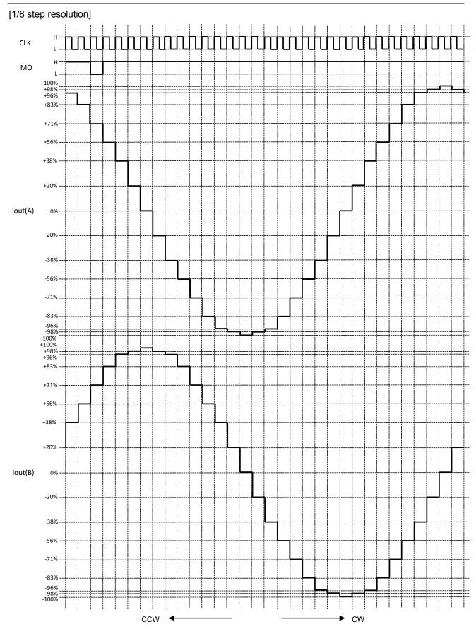
MO output shown in the timing chart is when the MO pin is pulled up.
