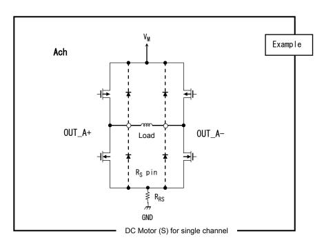
• ... Indicates an IC output pin connected to a motor.
