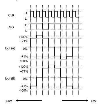
Note: MO signal is shown in the above timing chart when MO pin is connected with a pull-up resistor to VCC.
