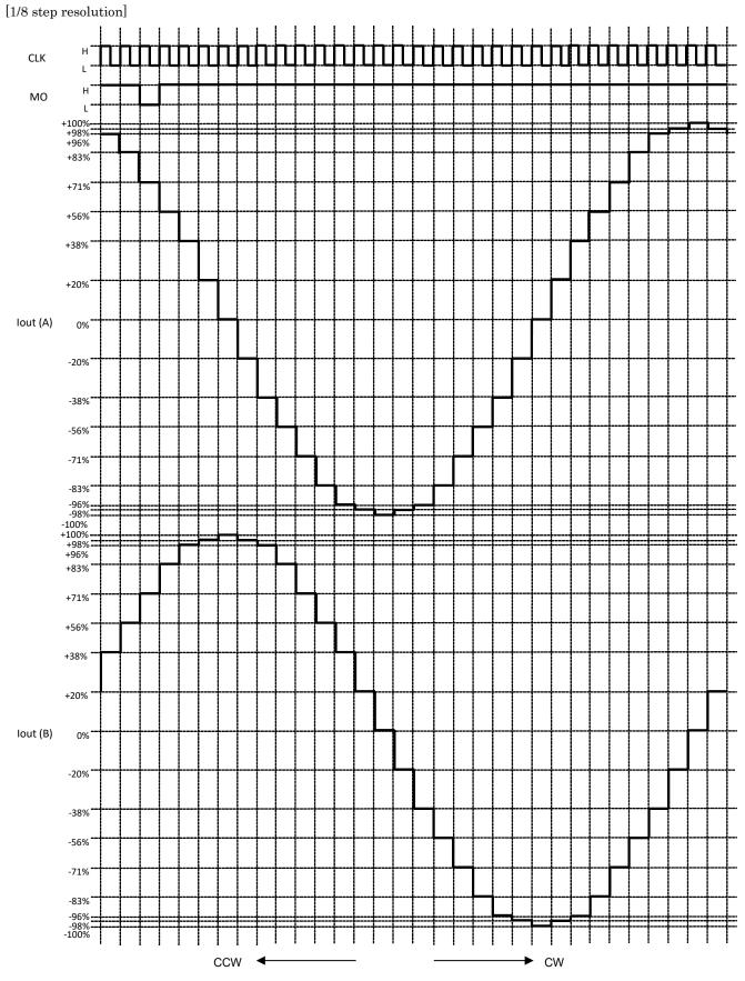
Note: MO signal is shown in the above timing chart when MO pin is connected with a pull-up resistor to VCC. Note: Timing charts may be simplified for explanatory purpose.
