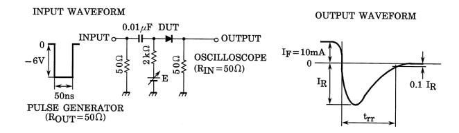
Fig.1 Reverse Recovery Time (t<sub>rr</sub>) Test Circuit
