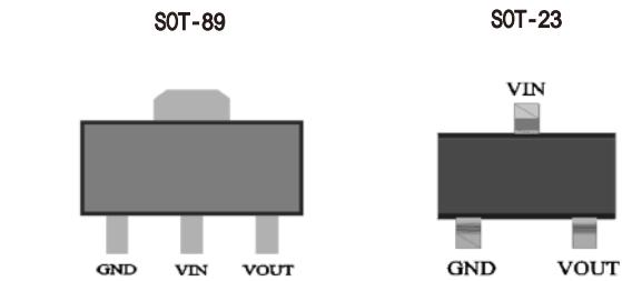
2.1V to 5.0V. CMOS technology ensures low voltage drop and low quiescent current.
