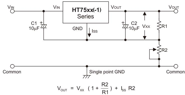
**Circuit for Increasing Output Voltage**
