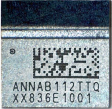
Figure 13: Product marking on the ANNA-B112 module
