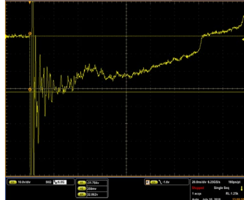
IEC 61000-4-2 -8 kV Contact ESD Clamping Voltage
