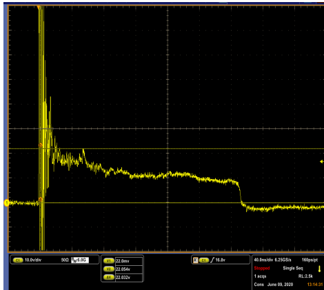
IEC 61000-4-2 +8 kV Contact ESD Clamping Voltage
