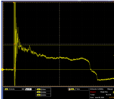
IEC 61000-4-2 +8 kV Contact ESD Clamping Voltage
