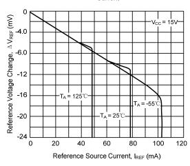
Reference Short Circuit Current vs. Ambient Temperature
