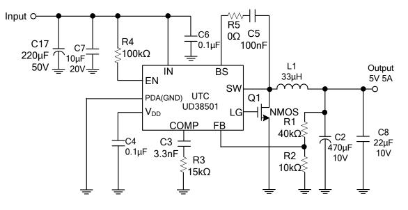
$V_{OUT}=V_{FB} \times (1+R1/R2)$ ,  $V_{FB}= 1.00V$ , R2 suggest  $10k^{\sim}30k\Omega$
