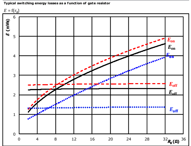
Figure 2. IGBT Typical switching energy losses as a function of gate resistor
