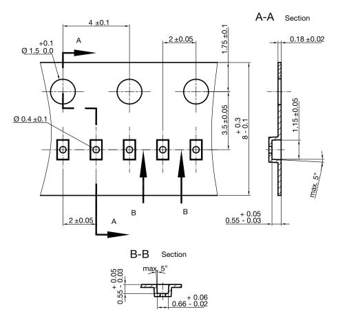
S8-V-3906.04-063 (4) created 28.10.2019 surface resistance:  $10^5 - 10^{11} \frac{OHMS}{SQ}$ Cummulative tolerances of 10 sprocket holes is ± 0.2 mm
