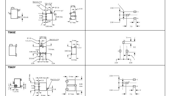
Three variations are available according to the positioning of the control screw and contact positions.
