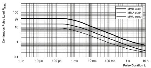
Maximum pulse load, continuous pulse; applicable if  $\overline{P} \leq P(\vartheta_{amb})$  and  $\widehat{U} \leq \widehat{U}_{max}$ ; for permissible resistance change  $\pm$  (0.5 % R + 0.01  $\Omega$ )
