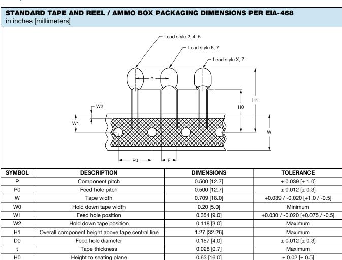
**Tape and Reel Packaging:** type 199D radial-leaded tantalum capacitors, all lead styles except 1, 3, and Y are available taped and reeled per EIA-468.
