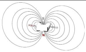
When a positive (+) voltage is placed on the terminal marked with the polarity dot and the opposite terminal is negative (-), the resulting current flow will create a magnetic south pole on the top side of the IHLP. Observing the polarity orientation when mounting the IHLP will insure the most consistent EMI reduction performance.
