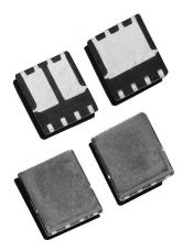
Figure 1. PowerPAK 1212 Devices
