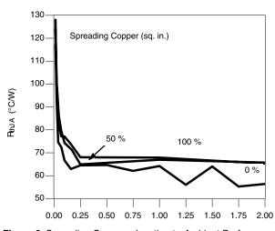
Figure 6. Spreading Copper - Junction-to-Ambient Performance
