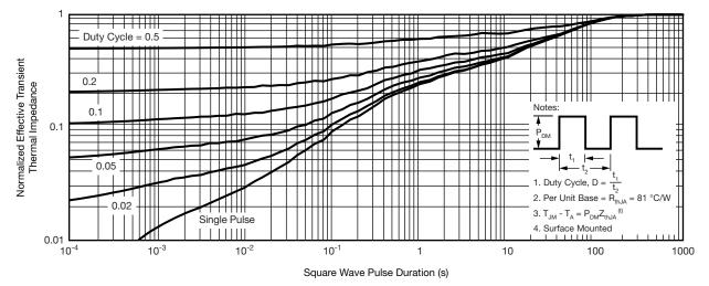
Normalized Thermal Transient Impedance, Junction-to-Ambient
