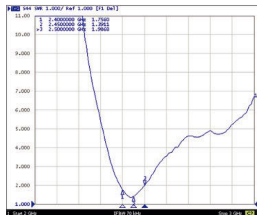
Antenna VSWR on Test Board
