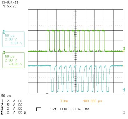
Green waveform: optical input signal to the photodiode that is connected to the amplifier circuit.
