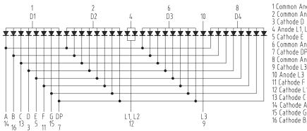
Common Anode 1 Common Anode D1 2 Common Anode D2 3 Cathode D 4 Anode L1, L2 5 Cathode E Common Anode D3 Cathode DP 8 Common Anode D4 9 Cathode L3 10 Anode L3 11 Cathode F 12 Cathode L1, L2 13 Cathode C 14 Cathode A 15 Cathode G
