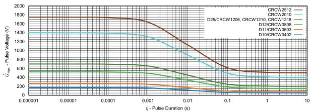
Maximum pulse voltage, single and continuous pulses; applicable if  $\hat{P}=\hat{P}_{\text{max.}}$ ; standard operation mode, for permissible resistance change equivalent to 8000 h operation
