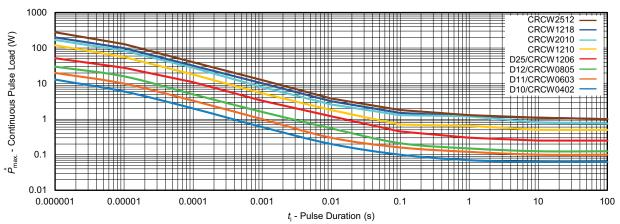
Maximum pulse load, continuous pulses; applicable if  $\overline{P} \le P$  ( $v_{amb}$ ) and  $\hat{U} = \hat{U}_{max.}$ ; standard operation mode, for permissible resistance change equivalent to 8000 h operation
