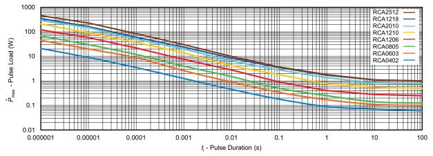
Maximum pulse load, single pulse; applicable if  $\overline{P} \to 0$  and n < 1000 and  $\hat{U} = \hat{U}_{\text{max}}$ ; for permissible resistance change equivalent to 8000 h operation
