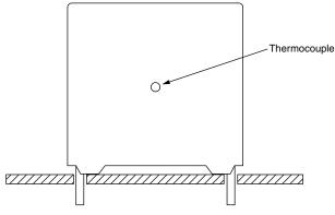
The temperature is measured in unloaded (T<sub>amb</sub>) and maximum loaded condition (T<sub>C</sub>). The temperature rise is given by  $\Delta T = T_C - T_{amb}$ .
