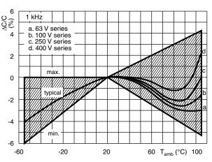
Capacitance as a function of ambient temperature
