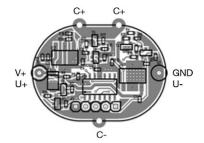
The arrangement of the cells is flexible. Usually, the firmware of the board is programmed specifically for a 196 HVC in the standard 90 F, 8.4 V configuration. Reprogram the controller for other voltages.
