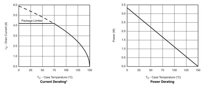
\* The power dissipation  $P_D$  is based on  $T_{J(max)} = 150$  °C, using junction-to-case thermal resistance, and is more useful in settling the upper dissipation limit for cases where additional heatsinking is used. It is used to determine the current rating, when this rating falls below the package limit.
