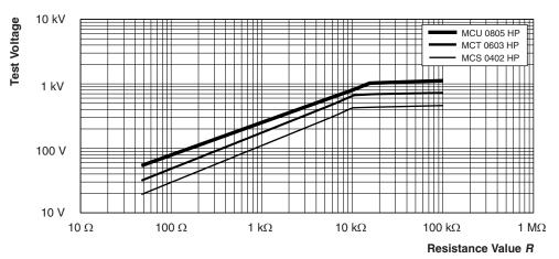
Pulse load rating in accordance with EN 60115-1 clause 4.27; 1.2  $\mu$ s/50  $\mu$ s; 5 pulses at 12 s interval; for permissible resistance change  $\pm$  (0.5 % R + 0.05  $\Omega$ )
