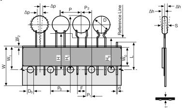
TAPING P / T / U COMPONENT PITCH 0.5" LEAD SPACING 7.5 mm
