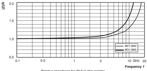
Relative impedance for 49.9  $\Omega$  chip resistor
