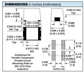
Recommended minimum spacing between components
