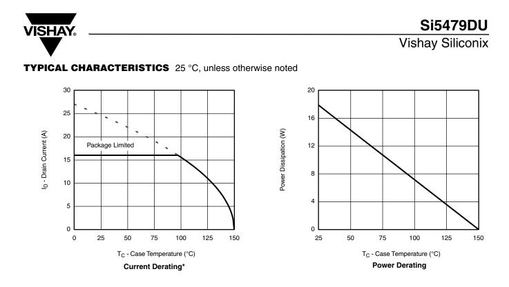
\* The power dissipation  $P_D$  is based on  $T_{J(max)} = 150$  °C, using junction-to-case thermal resistance, and is more useful in settling the upper dissipation limit for cases where additional heatsinking is used. It is used to determine the current rating, when this rating falls below the package limit.
