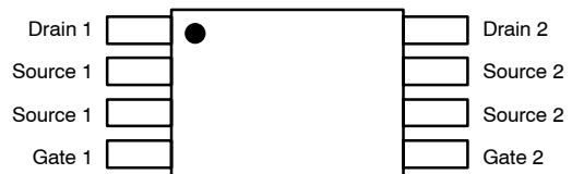
Figure 3. Pinouts for Dual-Die TSSOP
