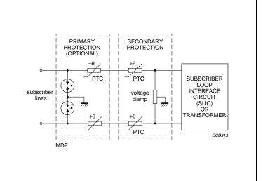
Fig.1 Typical telephone line equipment showing where PTC thermistors can be used for overcurrent protection.
