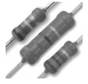
A homogenous film of metal alloy is deposited on a high grade ceramic body. After a helical groove has been cut in the resistive layer, tinned electrolytic copper wires are welded to the end-caps. The resistors are coated with a blue, non-flammable lacquer, which provides electrical, mechanical, and climatic protection.
