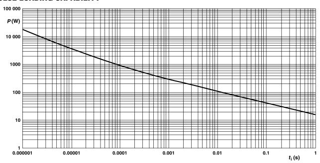
Pulse on a regular basis; maximum permissible peak pulse power  $(P_{max})$  as a function of pulse duration  $(t_i)$  for single pulse condition
