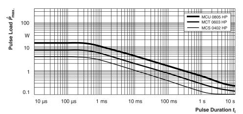
Maximum pulse load, single pulse; applicable if  $\overline{P} \to 0$  and  $n \le 1000$  and  $\hat{U} \le \hat{U}_{\text{max}}$ ; for permissible resistance change  $\pm$  (0.5 % R + 0.05  $\Omega$ )
