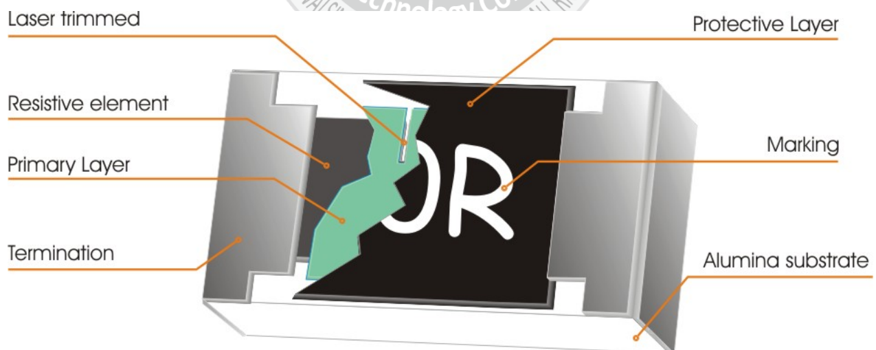
Fig 1. Construction of Chip-R SFxx_Q
