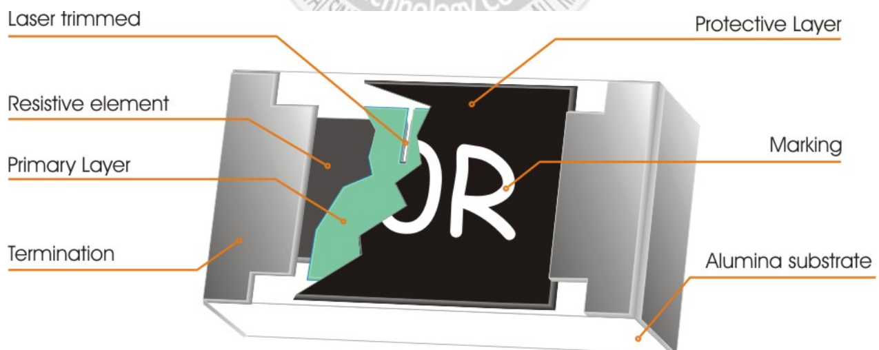
Fig 1. Construction of a Chip-R
