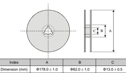
Note : The product shall be packed properly not to be damaged during transportation and storage. Taping Quantity : 3000 pieces per 7" reel
