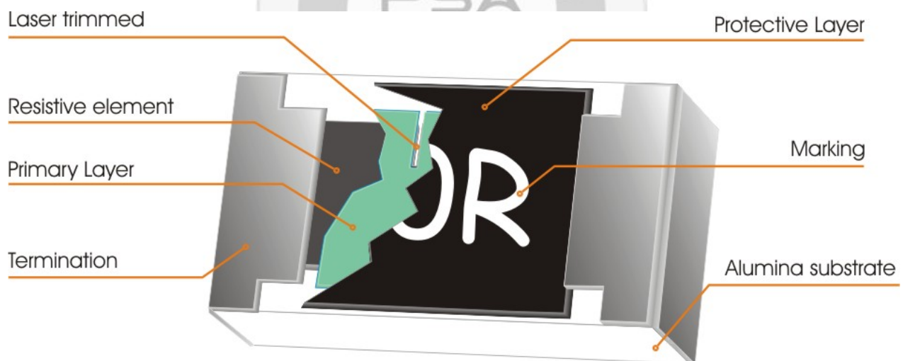
Fig 1. Construction of Chip-R
