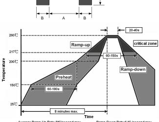
Average Ramp-Up Rate:3°C/second max. Ramp-Down Rate:6 °C /second max. Specifications are subject to change without notice.
