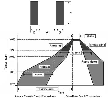
Notes: • If reflow temperatures exceed the recommended profile, devices may not meet the performance requirements.
