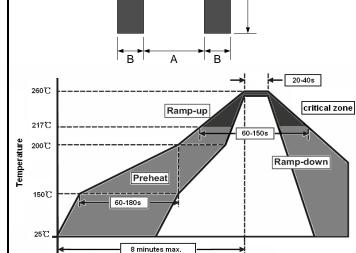
LP-NSM035/16 1.80 1.00 1.80 \* Recommended reflow methods: IR, Vapor phase, hot air oven.
