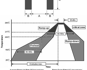
Average Ramp-Up Rate:3°C/second max. Ramp-Down Rate:6 °C /second max.
