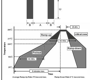
**Solder Pad Layouts** C Part number (mm) (mm) (mm)
